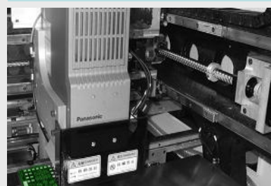
数字化控制X、Y轴运动 Digitally controlled linear axis for X & Y movement
