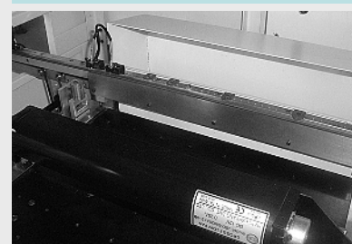
刻印除尘排风装置 Marking dust exhaust system
